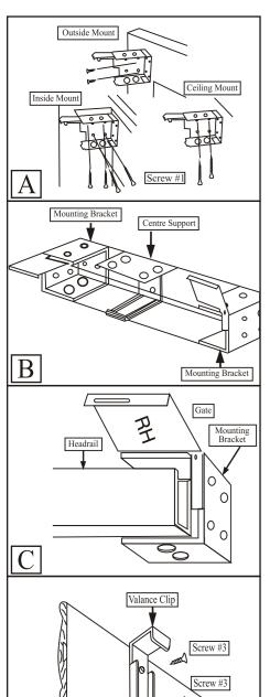
Brackets should be placed at the width of blind's head rail 6mm past each end. The bracket doesn't necessarily need to touch the inside face of the window frame.
