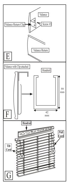
For Outside Mount: Screw one end of the valance return clip onto the valance using Screw #3. Align the edge of the valance return with the valance. Screw the other end of the valance return clip onto the valance return.
